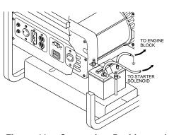
Figure 11 - Connecting Positive and Negative Cables to Battery (Model PGH7500IE Shown)
